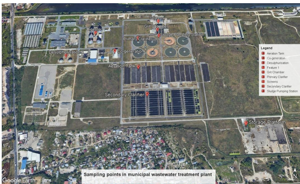
Fig. 3. The sampling points of the odour samples on the site of the municipal wastewater treatment plant
